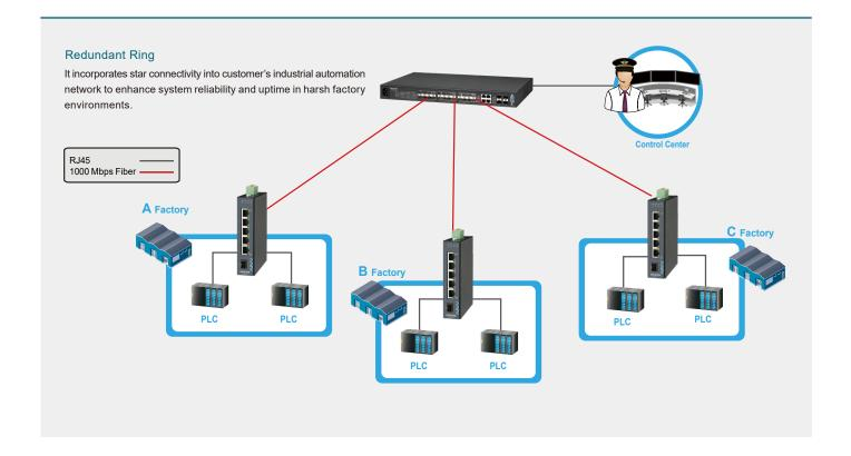
The INS-8615 is compatible with 10/100/1000Mbps through RJ45 transceivers to guarantee a strong & stable connection of Ethernet, Fast Ethernet or Gigabit Ethernet, providing flexible deployment options to satisfy industrial networking requirements
