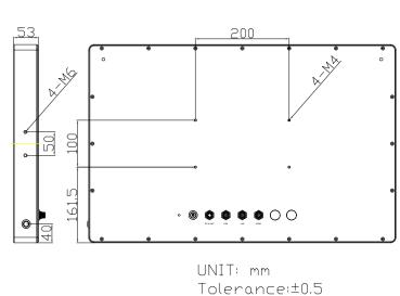
Mechanical 304 Stainless steel chassis(default), 316 Stainless steel Construction chassis(optional) Mounting VESA mount 200 x 100, Yoke mount for optional Total IP66/IP69K IP Rating Dimensions 656 x 423 x 53 mm 12.6 kg Net Weight
