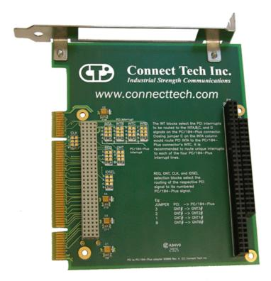
This passive extender card allows developers to mount a PCI-104 or PC/104-Plus card into a Universal PCI bus system. The adapter is equipped with a stack-through connector so the test card can be installed on either side, enabling probing on the front or the back (model AD001). The design also allows cables to exit from the host PC for easy connection to external devices.
