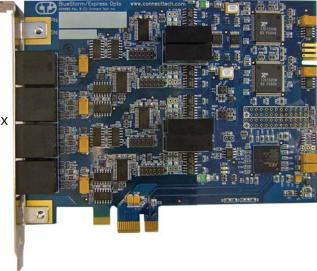
An extension to the BlueStorm/Express product family, the BlueStorm/Express Opto offers dependability and high speed data transfer rates along with 3kV optical isolation. This protection makes PCI Express Opto cards ideal in environments where harsh conditions may disrupt communications.
